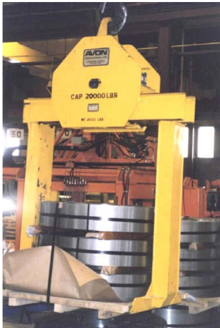
Telescopic pallet lifter Whether motorized or manual, telescopic pallet lifters handle palletized slit coils.
