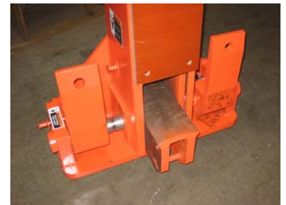
Coil lifter down, pallet forks up
