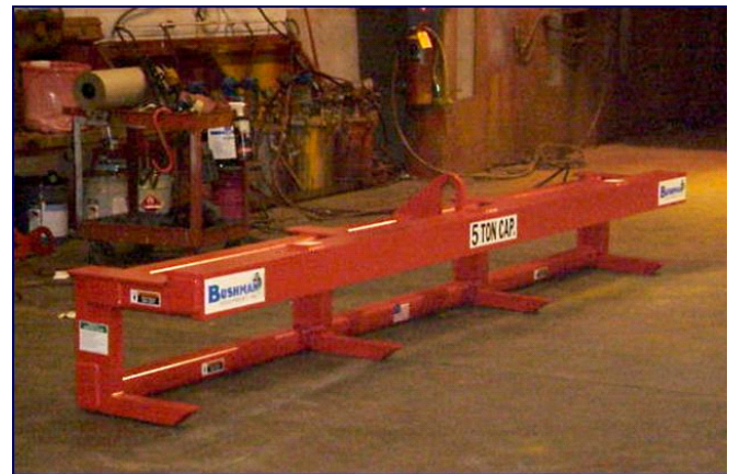
Pallet lifter modified to lift billets
