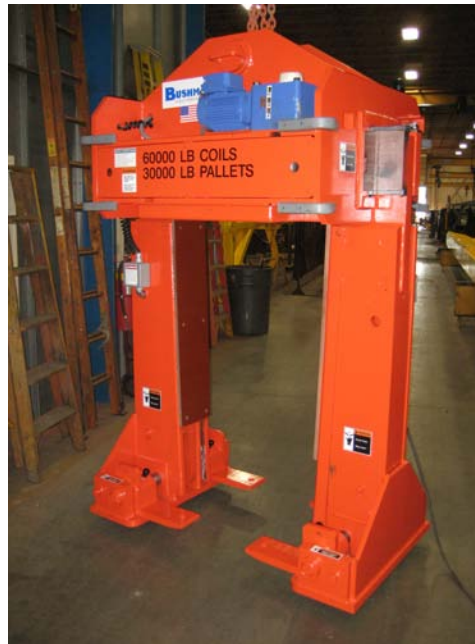
Combination coil/pallet lifter A Mexican steel maker purchased five combination coil/pallet lifters. They can lift 30-ton coils eye-horizontal or up to 15-ton coils on pallets eye-vertical.
