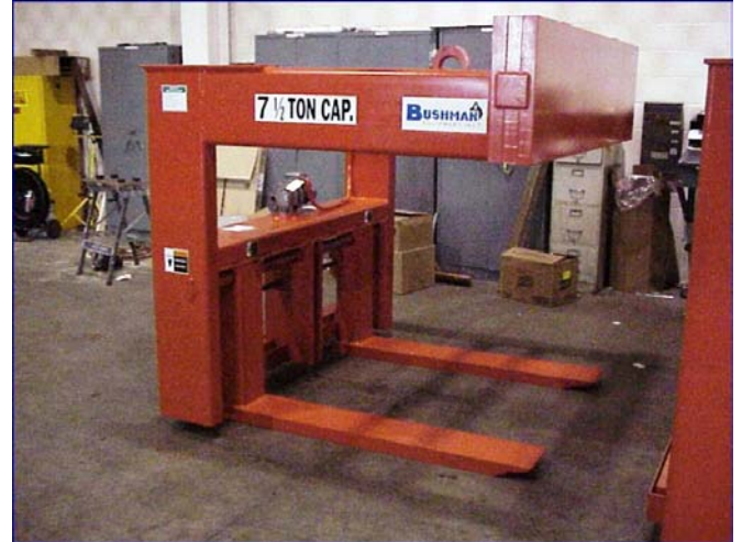
An electric motor adjusts the forks on this lifter
