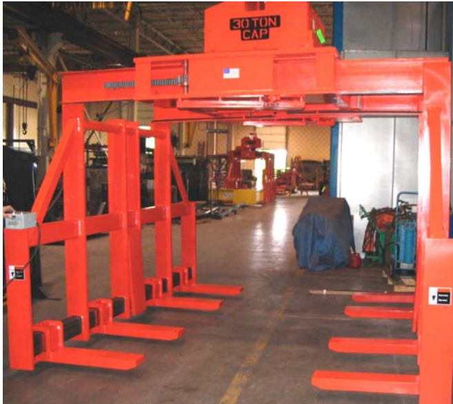
This motorized 30-ton capacity unit lifts pin-pallets for an auto maker. It has adjustable forks and motorized rotation.
