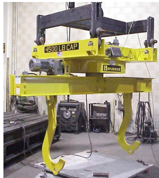
This rotating beam has adjustable J-hooks and an integral weigh scale system.
