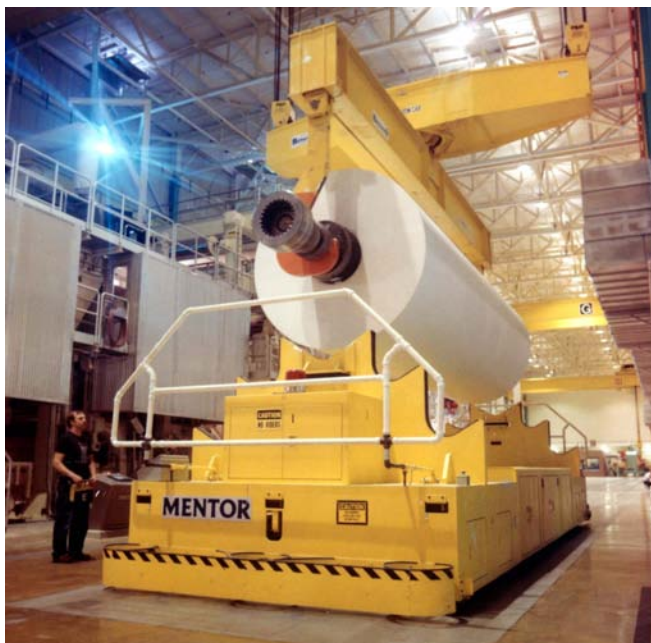
Rotating spreader beam in use at a paper mill.
