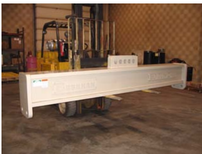
This extreme low temperature beam is made from special steel.
