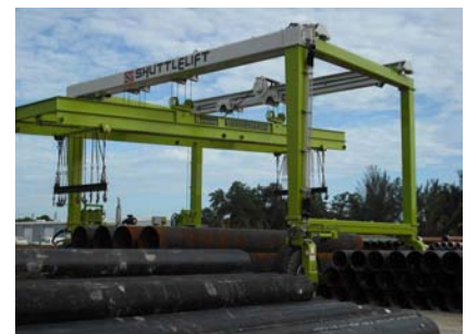
Beam with hydraulically adjustable lifting hooks
