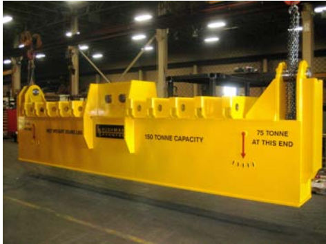
This 150 metric ton capacity spreader beam uses nylon straps positioned at multiple locations. It is designed for use with a single crane with a two-pronged hook or with two cranes, one attached to each end of the beam. The beam has load level indicators on both ends and both sides.
