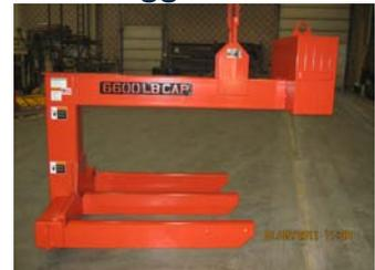
Designed for lifting three hot forgings at once
