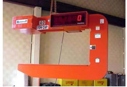
Bushman C-hooks can also be equipped with integral load weighing systems. The accuracy of the load cells is from plus or minus 0.2% to 0.5% of full load. The calibration settings are saved in memory even during loss of power. All Bushman C-hooks are designed and manufactured in accordance with ASME Spec. B30.20 and BTH-1: Design of Below-the-Hook Lifting Devices.
