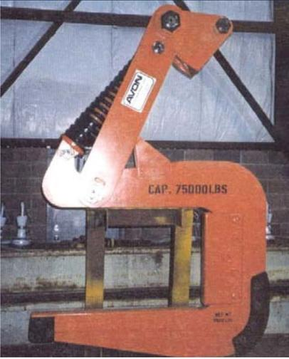
Spring balanced C-hooks are particularly useful for handling large coils. By eliminating the need for a counter weight, they minimize the weight of the hook. Coil edge protection is available.
