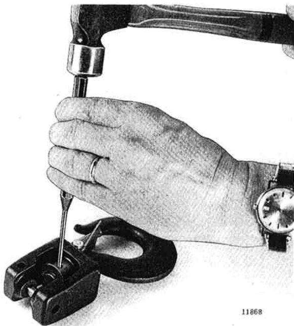
Figure 7-26. Removing Roll Pin Securing Hook Nut to Hook Shank.
