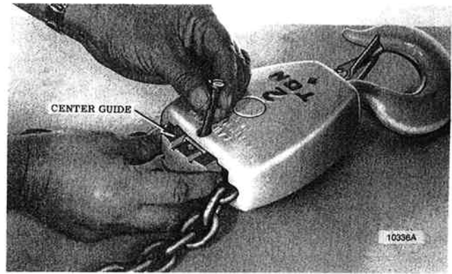
Figure 7-27. Removing Chain Center Guide from 2 thru 5 Ton Lower Block Assembly (Link Chain Model).
