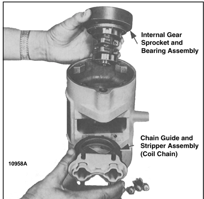
Figure 7-12. Removing Internal Gear, Chain Sprocket and Ball Bearing Assembly (Coil Chain Model).
