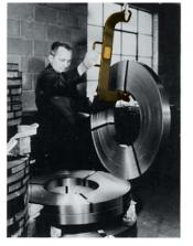
Coil is in vertical position after being lifted from its pallet. The weight of the coil holds the pivoting wedge in the vertical position during transportation.
