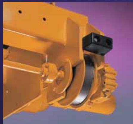
Totally enclosed, heavy-duty oil bath lubricated trolley traverse drive turns two rotating axle wheels connected by a line shaft. All wheels are supported on both sides by anti-friction bearings.
