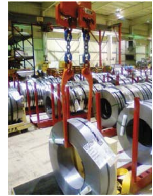
Once between the coils, legs will rotate 90 degrees.
