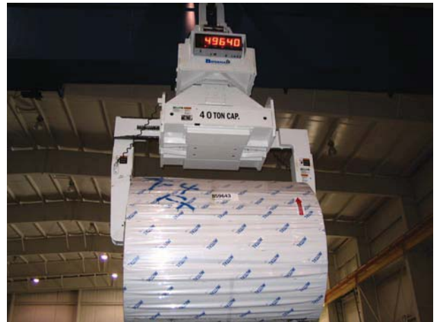
Bushman coil lifters can be equipped with weighing systems to weigh coils during the lift. This saves time by not having to use a separate floor scale.
