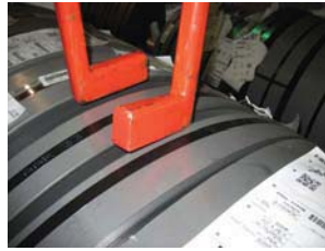
Coil lifter legs ready to slip between coils
