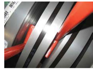
Once between the coils, legs will rotate 90 degrees.
