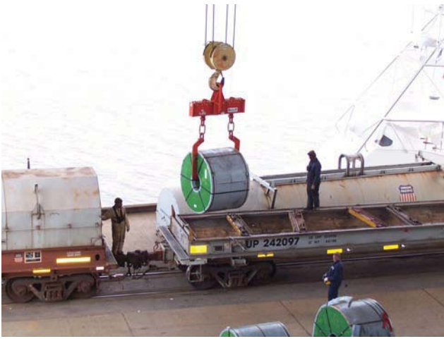
This 25-ton capacity adjustable coil lifter is offloading steel coils from a railroad car in Houston.
