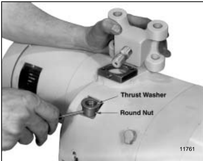
Figure 7-20. Removing Suspension Lug (1/4 thru 1 Ton Models)
