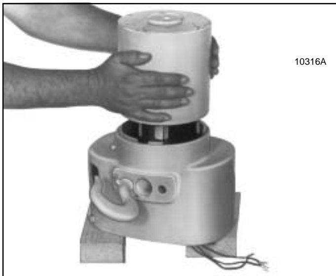
Figure 7-9. Removing Motor Assembly
