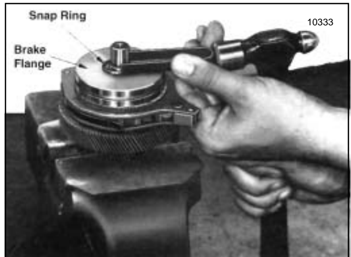
Figure 7-21. Removing Snap Ring from Load Brake Shaft
