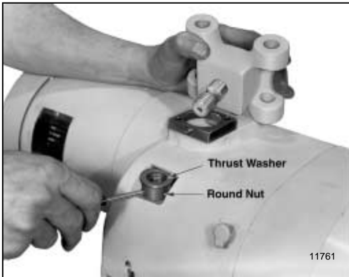
Figure 7-20. Removing Suspension Lug (1/4 thru 1 Ton Models)
