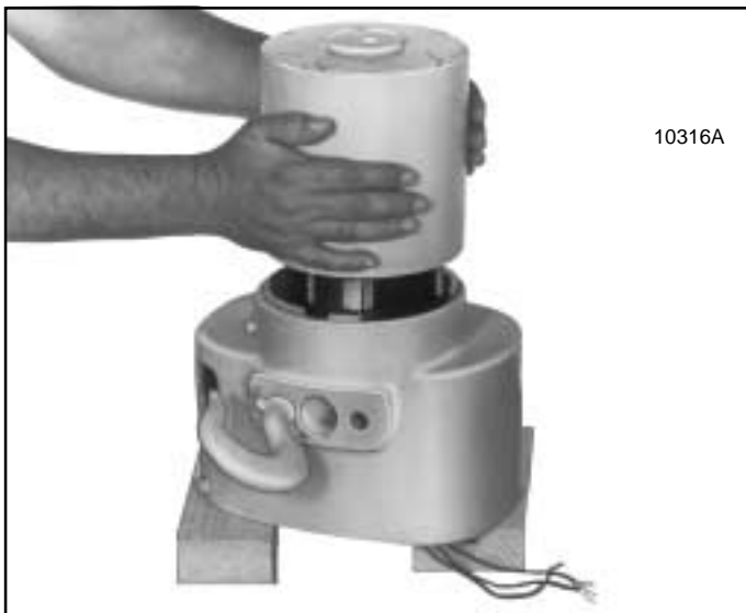
Figure 7-9. Removing Motor Assembly
