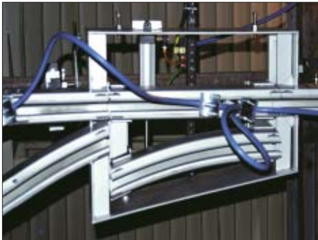
Powered track switch for use in monorail applications
